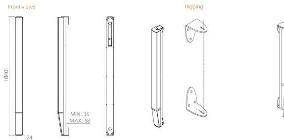
Mount the column using the supplied nut and screw
