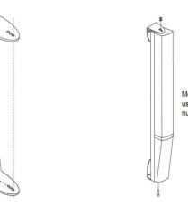
Mount the column using the supplied nut and screw
